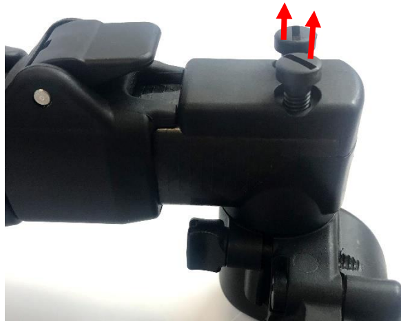
Figure 48: Remove Screws from Lower Shaft
