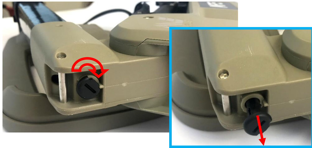
Figure 47: Remove Pin Coil Cable from the upper shaft
