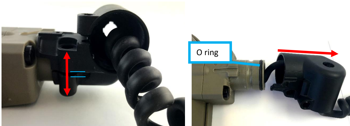
Fig 55: Remove Pivot Coil Yoke
