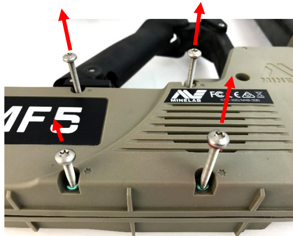
Figure 12: Remove four (4) Screws Torx T20
