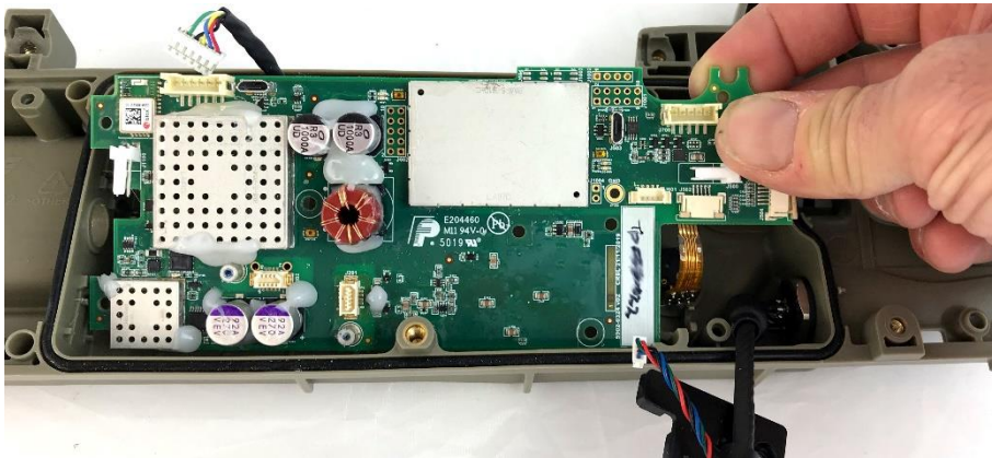
Figure 36: Insert Main PCB
