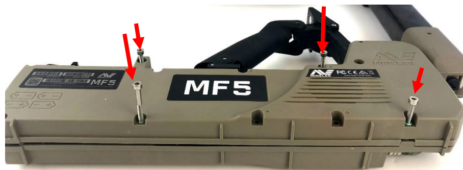
Figure 21: Insert Four Screws
