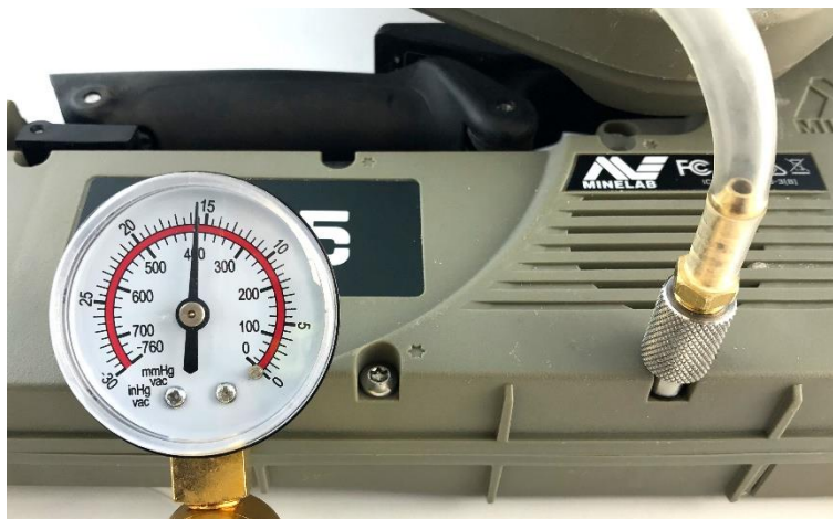
Figure 112: Apply a vacuum of 50kPa
