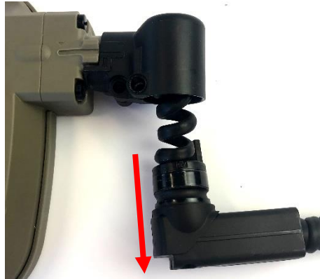
Fig 54: Remove Pivot Lower
