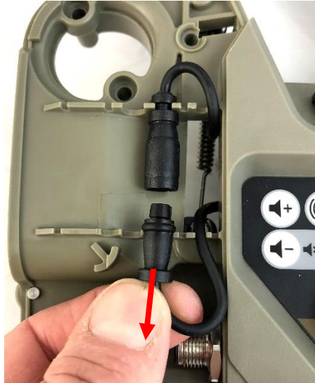
Figure 77: Disconnect Wiring Loom Handle
