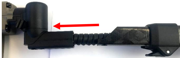
Figure 75 Remove Coil Cable from Shafts
